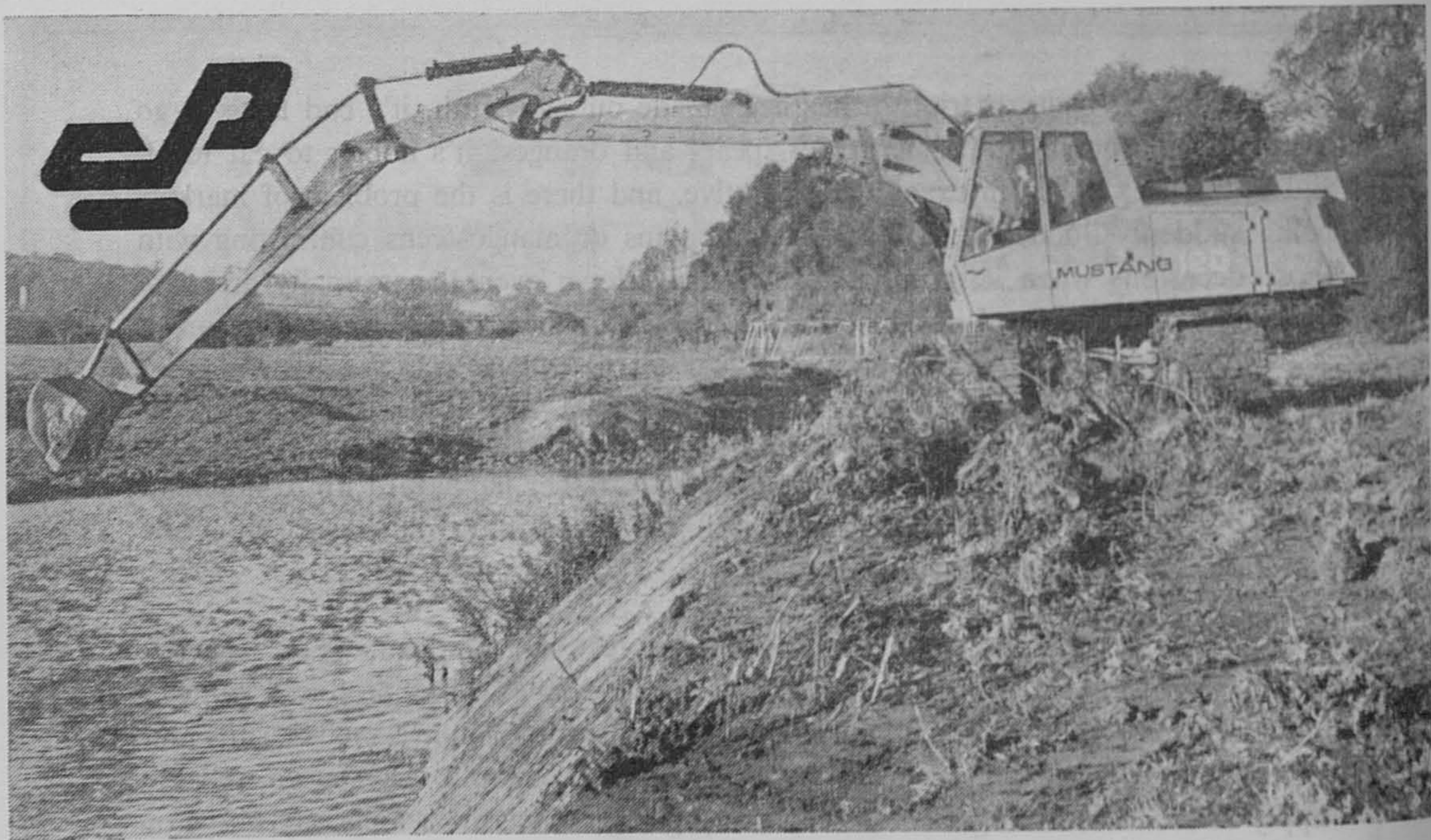
MUSTANG 120 DITCHING TO 35' 0" (10.7m)
