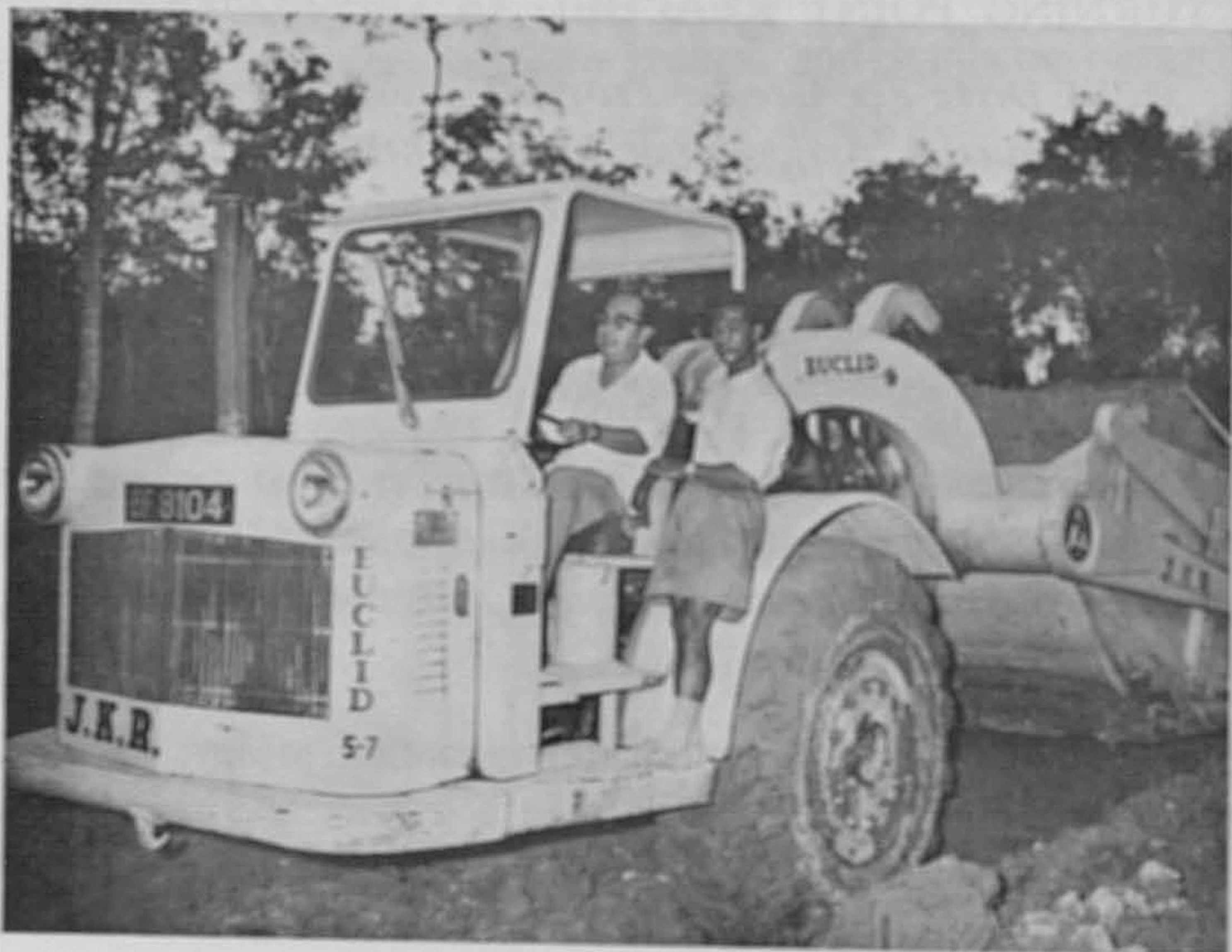
The Tun is driving a Euclid TS-7 self-propelled scraper when he inspected the progress of Padang Tengku Road, Kuala Lipis, Pahang, on 15th December, 1961.
