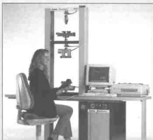
Zwick 1446 Universal Testing Machine with a table on which to place specimen
