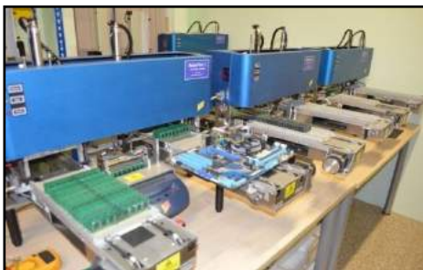
Syarikat Mushkin Sdn.Bhd., Kuala Lumpur - RoboFlex III Pick & Place Handler Robotic Memory Testing System (10.04.2013)
