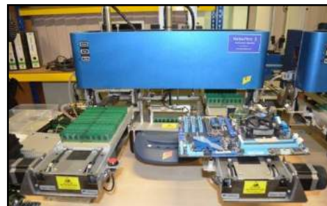
Syarikat Mushkin Sdn.Bhd., Kuala Lumpur - RoboFlex III Pick & Place Handler Robotic Memory Testing System (10.04.2013)
