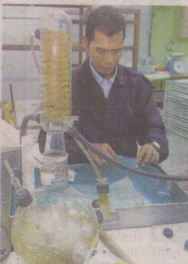
2. The documents are soaked in a solution of distilled water and magnesium carbonate for 45 minutes to rid it of acid.
